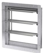
The WD-320 series dampers are designed to prevent reverse airflow in horizontal exhaust applications. The WD-320 features a pressure sensitive blade design that opens and remains open under low velocity conditions. The dampers are opened by air pressure differential and closed by gravity. Galvanized steel frame with flange on the discharge side.
